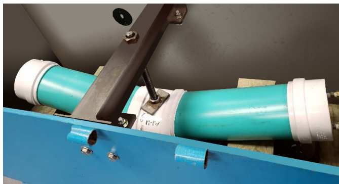
Figure 3 – Example of Angular Joint Deflection Setup for Pressure and Vacuum Tests for standard sewer fitting
