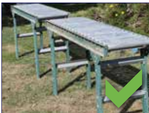
Pipe roller table setup
