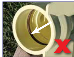
O-ring in spline groove
