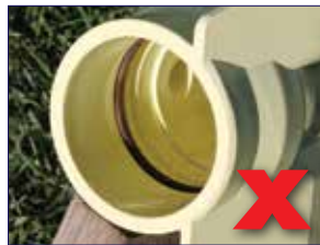
O-ring in spline groove
