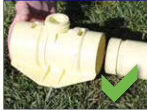
Properly aligned pipe and sled coupling
