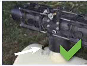
Secure Nelson valve installed onto tapped coupling with spline
