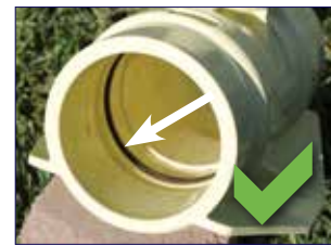
O-ring properly installed
