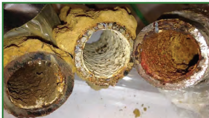
FIGURE A.25 : CORRODED IRON PIPE SAMPLES FROM FLINT, MI
